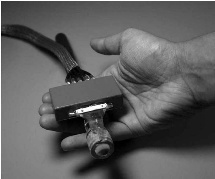
Figure 2. Photograph of a prototype annular array and flex circuit containing the electronic fan-out.
